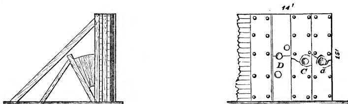
Side and front of 6½-in. laminated target.
