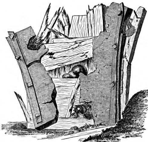
4½-in. plate, faced with 4-in. rubber, after three 11-inch shot.
