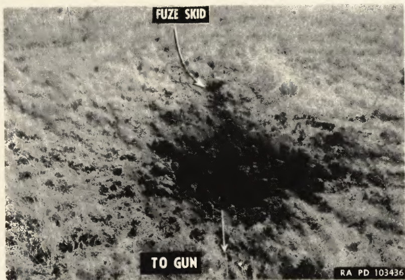
Figure 1—Shell Crater With Fuze Skid
