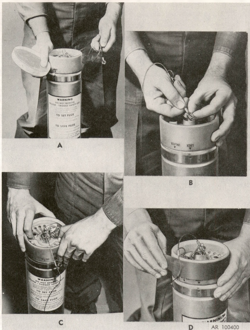
Figure 2-1. Attaching lanyard and setting fuze.
