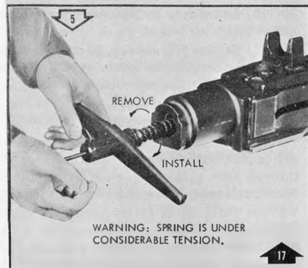
E. SPRING DISMANTLING DEVICE.
