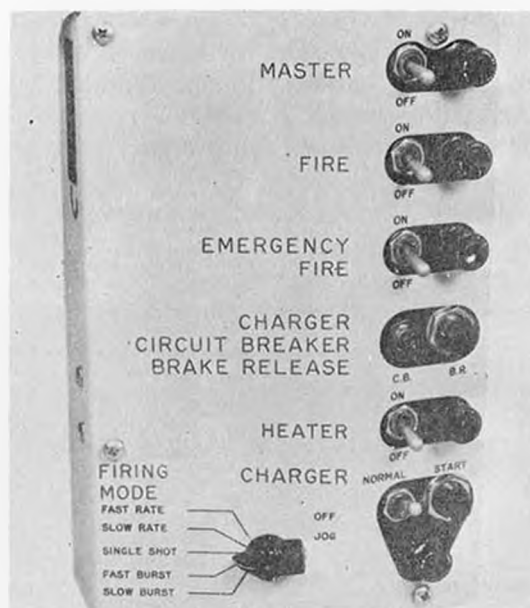
Figure 6. Fire control box.
