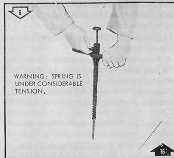
F. REMOVE/INSTALL DRIVING SPRING GROUP.
