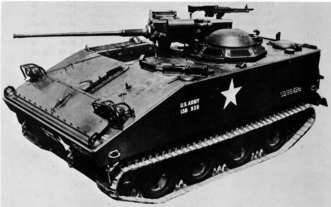
Figure 1. Carrier, Command and Reconnaissance: Armored M114A1E1— left front view.
