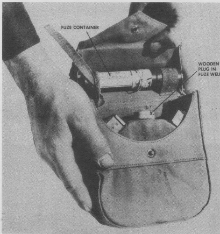
Figure 9. Canvas carrying pouch for magnetic mine.
