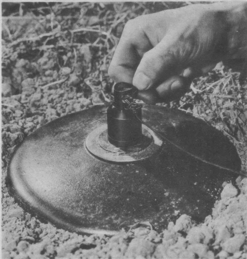
Figure 23. Removing safety pin from safety-pin hole of fuze.
