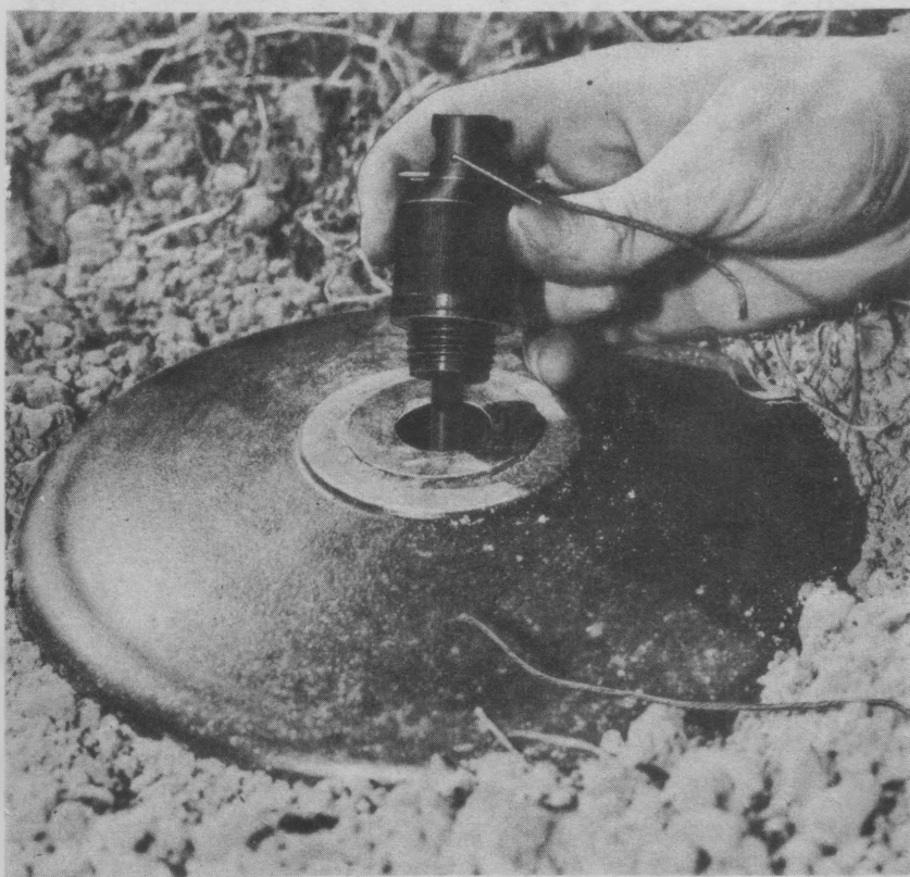
Figure 24. Defuzing type 3 land mine.
