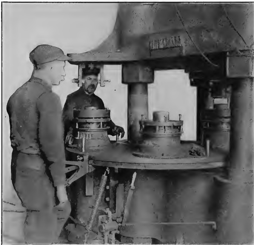
FIG. 5. HYDRAULIC HEADING PRESS FOR 4.5 CARTRIDGE CASES
