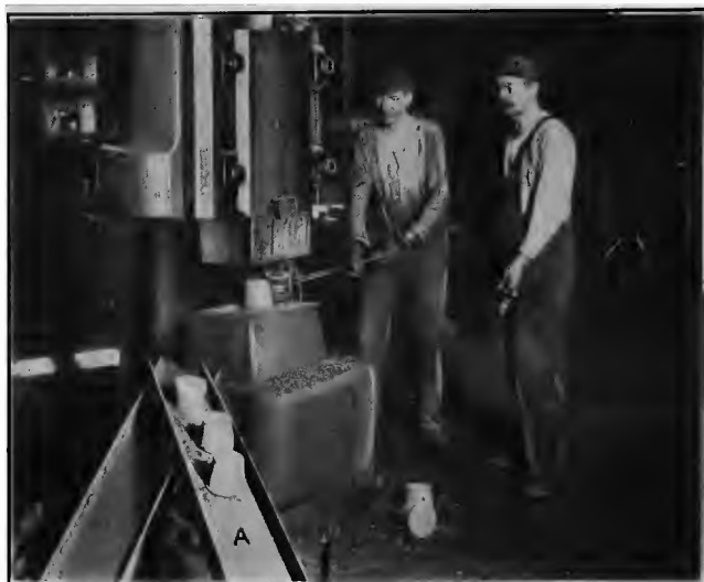
FIG. 4. UPSETTING THE BLANKS
