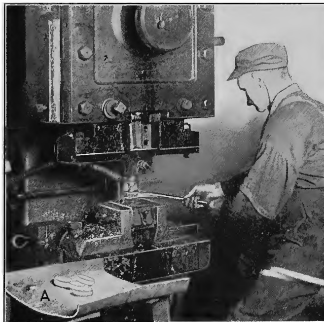
FIG. 3. DEEPENING THE DISKS
