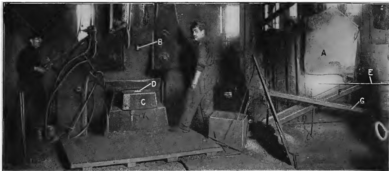
FIG. 5. FIRST AND SECOND PIERCING OPERATIONS
