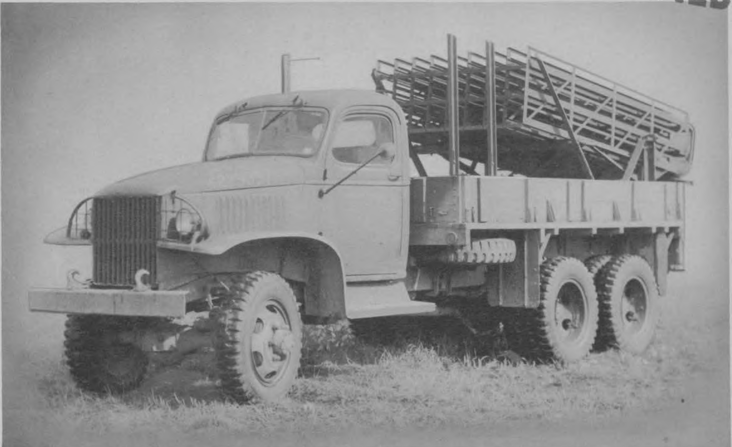
7.2 INCH MULTIPLE ROCKET LAUNCHER, T32, MOUNTED ON 2 1/2-TON TRUCK
