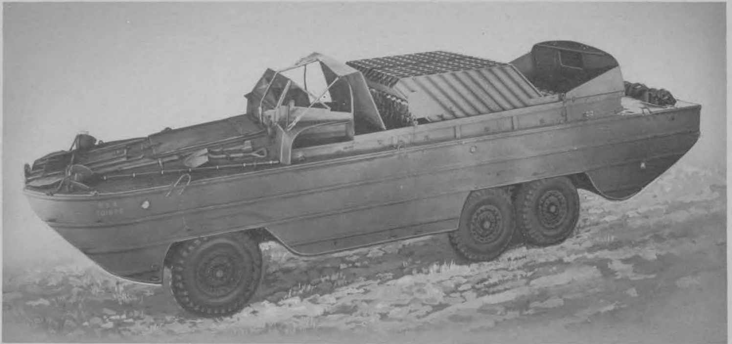
4.5 INCH MULTIPLE ROCKET LAUNCHER, T44, INSTALLED IN AMPHIBIOUS TRUCK
