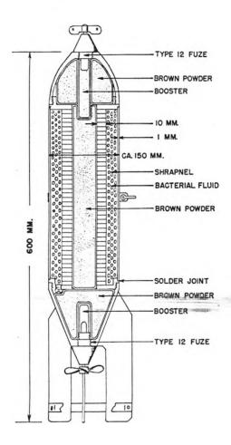
PRODUCTION: 300 ROUNDS IN 1938 WEIGHT: 40 KG. CAPACITY: 700 CC. BACTERIAL FLUID-1500 STEEL PELLETS FUZES: TYPE-YEAR 12 "TOKA SHUNPATSU" EXPLOSIVE: APPROX. 3 KG. BROWN POWDER (TNT)
