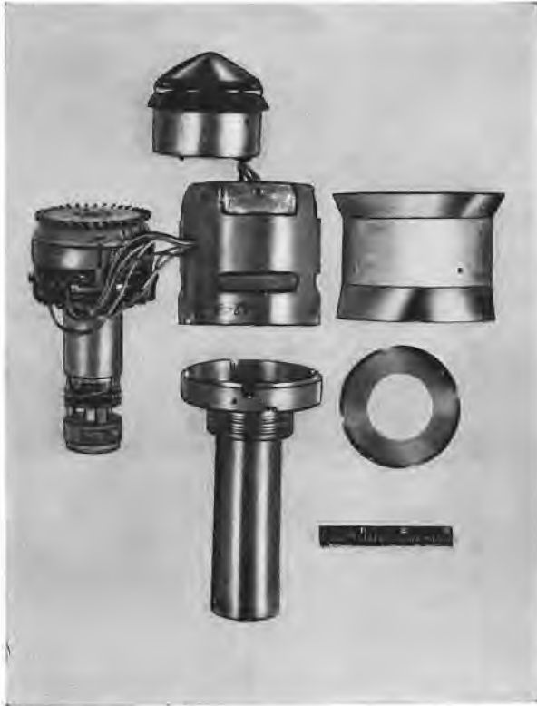
FIGURE 13. Photoelectric generator-powered bomb fuze, BPEG, disassembled into principal subassemblies. At top, electronic unit, with photocell and lens. At left, power supply, arming and detonator assembly. At center, unit housing. At right, air director cowl. Below, unit base housing and, at right, insulating washer. (Photograph by Bell Telephone Laboratories.)
