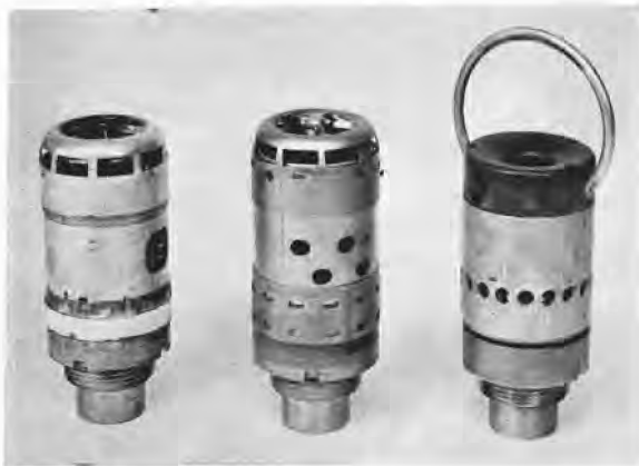
FIGURE 5. Radio proximity fuzes for trench mortar shells. These are, from left to right, T-132, T-171, and T-172. The first two use the missile as an antenna, and the last carries its own antenna in the form of a loop.
