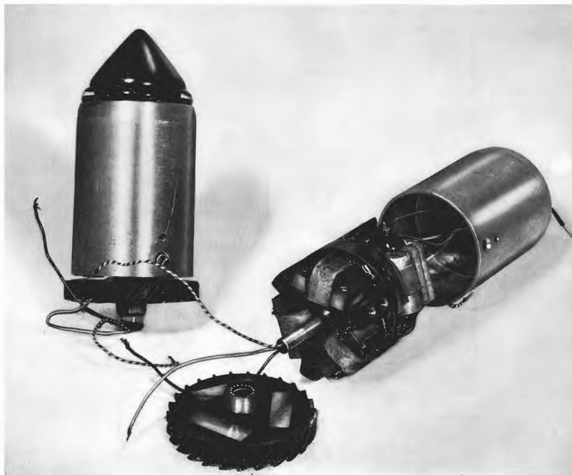
FIGURE 12. Photoelectric generator-powered rocket fuze, RPEG. At left, electronic and power supply assembly. At right, unit disassembled to show electronic and generator stator subassembly and turborotor. (Note detonator leads which are fed through hollow shaft.)
