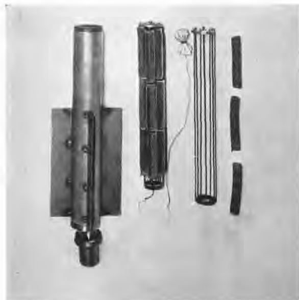
FIGURE 1. Test rocket (3.25 in.) showing motor body with fins attached and nozzle directly below. Loaded power cage, black powder igniter with enclosed electric detonator, bare wire cage, and representative samples of propellant are also shown.
