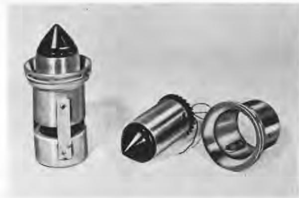
FIGURE 11. Photoelectric generator-powered rocket fuze, RPEG. At left, experimental model with improvised housing for arming switch SW-200 attached at rear. At center, electronic and power supply assembly. At right, cowling member for directing air to and from turbine.
