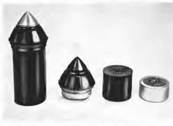
FIGURE 2. T-4 photoelectric fuze, developed for use on M-8 rocket. From left to right are shown: assembled fuze ready for installation in rocket; MC-380 nose containing electronic control elements; BA-75 battery; and SW-230 switch. Nose and switch plug into opposite ends of battery.
