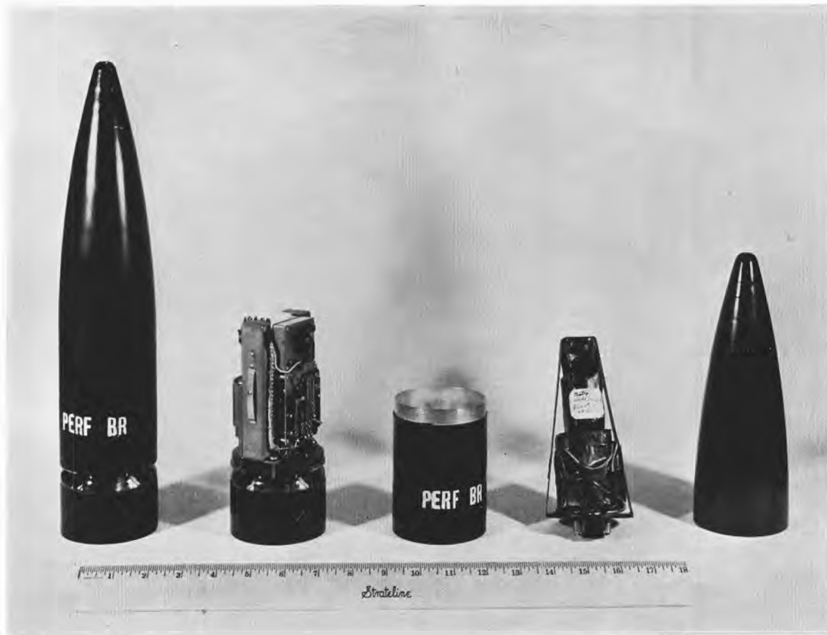
FIGURE 3. Model BR photoelectric rocket fuze. Left, completely assembled fuze ready for installation on rocket. Next, from left to right, electronic assembly showing arming switch, cylindrical housing, battery, and rocket ogive which encloses battery.
