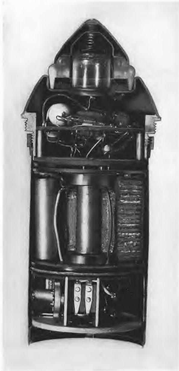
FIGURE 4. Cutaway of T-4 photoelectric fuze showing placement of components.
