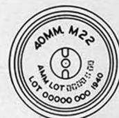
REAR FACE OF M22 CASE W/PRIMER MK.I/L.
