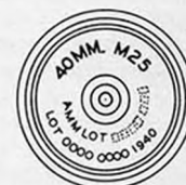
REAR FACE OF M25 CASE W/PRIMER M23A2
