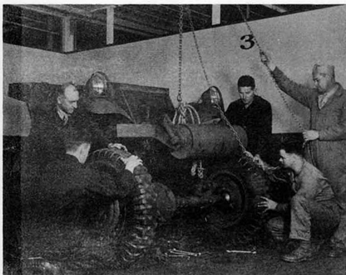
Students receive special instruction in assembly, alignment, and adjustment of front wheels at the Cleveland Section.
