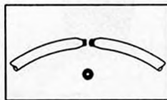
Cup-and-cone break, no abrasion
