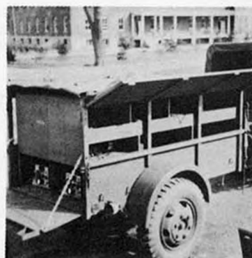
Rear view showing storage compartments for two (2) complete burners
