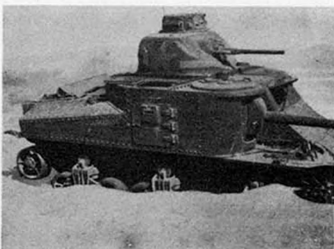
M3 tank digging in on towing without a track
