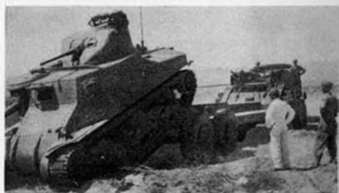
Above: The tank approaches the trailer, and below: it is drawn onto the trailer by cables
