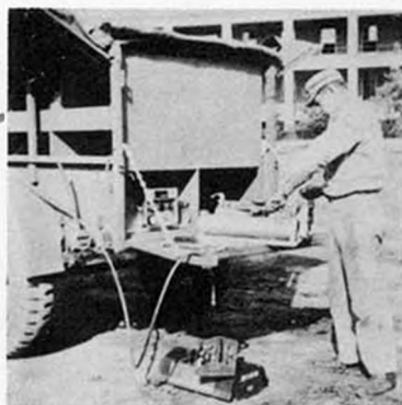
Rear view showing mechanic making repairs using tail gate as a work bench
