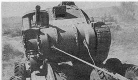
Above: Tractor of T-3 unit using winch to tow tank in difficult terrain. Below: The tank being towed.
