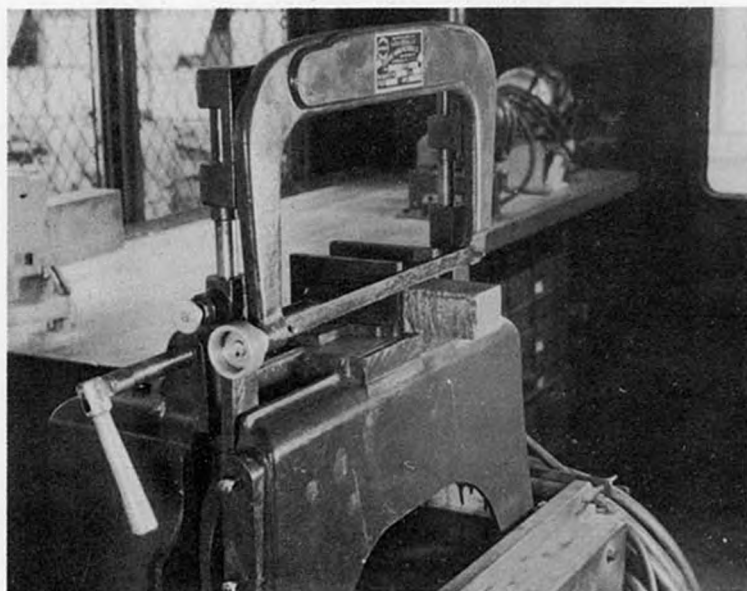
Figure 21 -- Cutting metal section with power hacksaw on M3 welding truck
