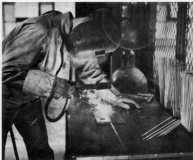
Figure 7 -- Electric arc welding on M3 welding truck
