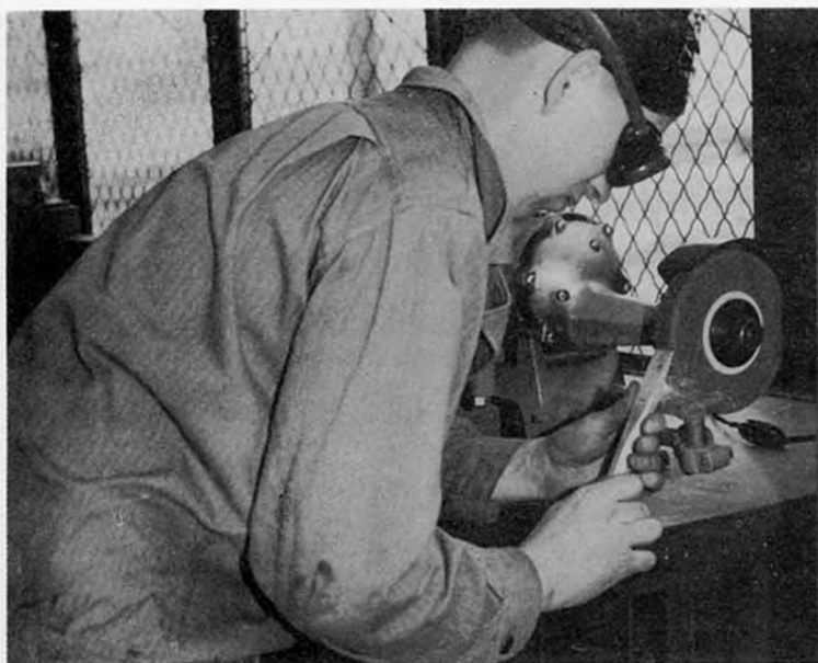
Figure 19 -- Sharpening chisel by grinding, using portable electric grinder mounted on bench stand, M3 welding truck
