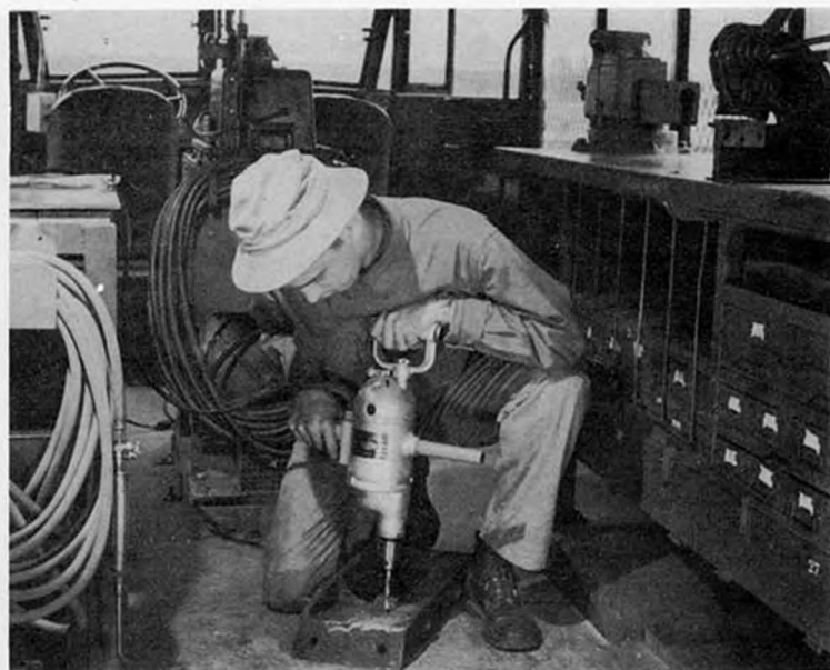
Figure 20 -- Drilling web section of welded section, using portable electric drill, M3 welding truck
