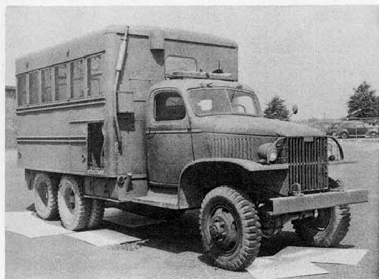
Figure 28 -- Truck, welding, M12 (right front view)
