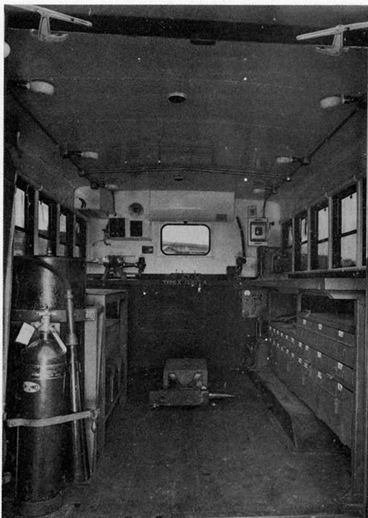
Figure 32 -- Interior view of welding truck M12, showing anvil and block in traveling position
