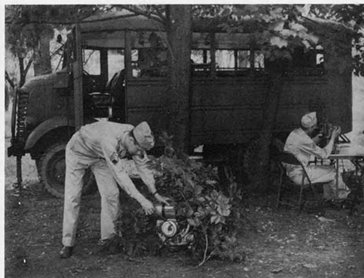
Fig. 5 -- A portable generator is furnished for use when current cannot be obtained from the machine shop truck or an outside source. The generator shown above is a portable, 1-1/2 KW, 110-volt, 60-cycle, AC, gas engine driven generator. It is small, compact and easily concealed for use.
