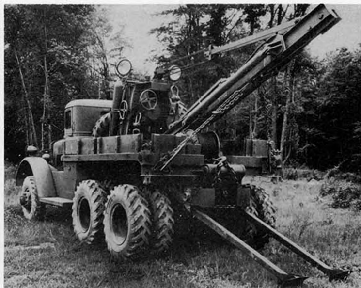
Figure 4 Wrecker in position for rear recovery operation with spades out.
