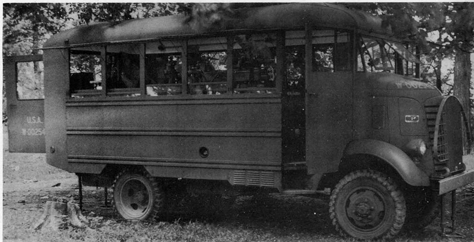
Fig. 2 -- The Instrument Repair Truck, M1, with stabilizing jacks in place; windows open, and grating up; rear door open. Optical instru-
