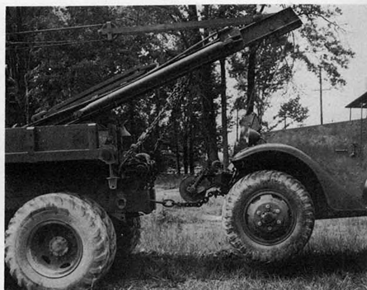
Figure 9 Towing hookup that may be used to tow a wheeled vehicle with a damaged front drive. This hookup is especially suitable for crossing rough terrain.
