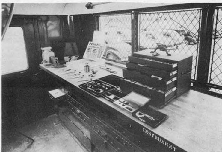
Fig. 14 -- Showing an instrument kit partially open, and beside it, some of the many precision measuring and other tools, comprising the equipment of the instrument truck.
