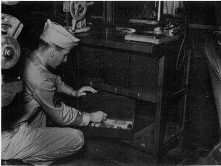
Fig. 8 -- In addition to the large number of tools and other equipment on the truck, four complete kits for instrument repairmen are included. These kits form a complete working set of tools for inspecting and maintenance parties on detached missions, as well as being of valuable use to supplement the equipment on the truck.
