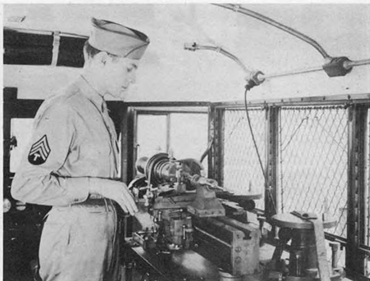
Fig. 13 -- One of the most important items of equipment on the truck is the precision bench lathe, back geared, screw cutting, 8-1/2 x 40 inch, with 1-inch collet capacity, quick change gear box, taper attachment, 1750 r.p.m., 3/4 hp., 110-volt, 60-cycle, single-phase AC, repulsion induction motor with reversing switch, complete with all necessary accessories for extensive field maintenance operations.
