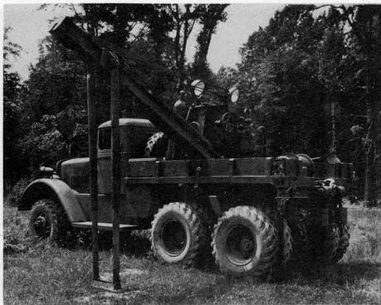
Figure 5 Wrecker with boom swung out laterally, A-Frame down and body jacks in place.
