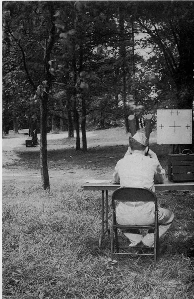
Fig. 7 -- Most operations involving optical instruments require that testing targets be at a given distance. In certain operations, such as
