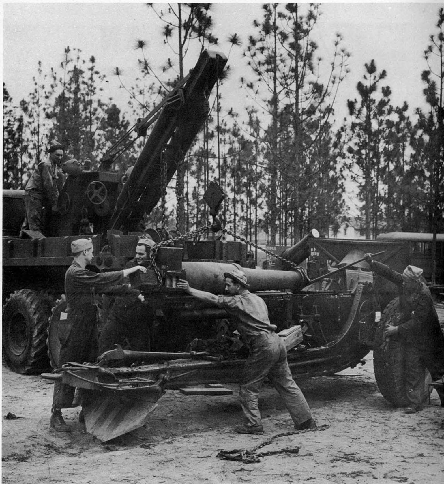
Removing tube from cradle of 155mm Howitzer (113th Ord. Co.)
