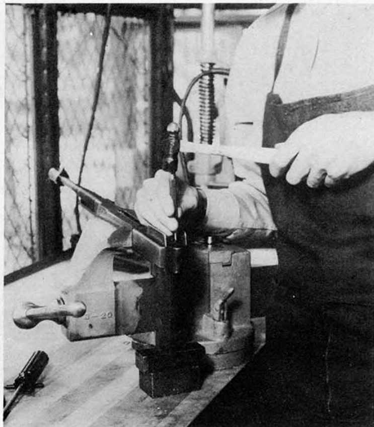
Fig. 3. Removing and replacing an unserviceable rear sight fixed base.
