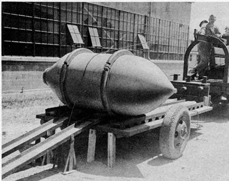
The bomb is rolled on to the trailer by use of the winch to this point, and from here on it is rolled by hand. Note: the shipping bands are around the outside of the two center channels.
