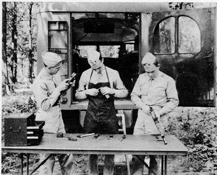
Fig. 1. -- Left to right: H. L. Bagley, 2nd Lt., Ord. Dept., Checking the frame group mechanism; A. C. Fabrize, T. Sgt., Ord. Dept., Reshaping the lips on a magazine; J. E. Johnson, 2nd Lt., Ord. Dept., Assembling recoil spring, buffer pilot and pad in the receiver.
