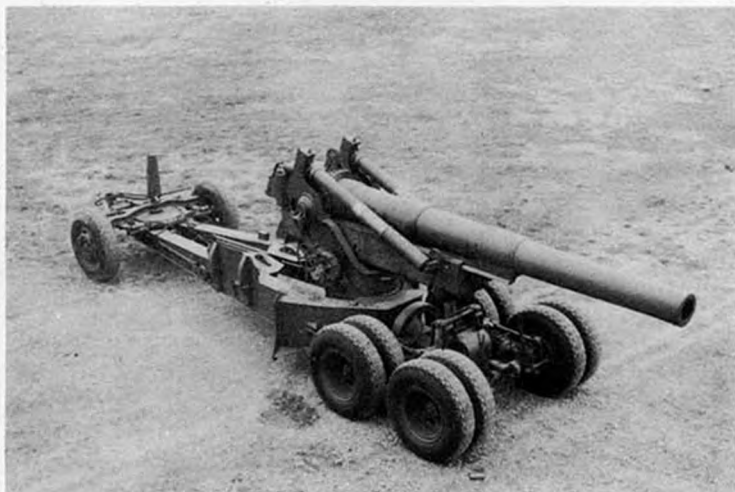
8" Howitzer, M1, on 8" Howitzer Carriage, M1, in traveling position without cover.
