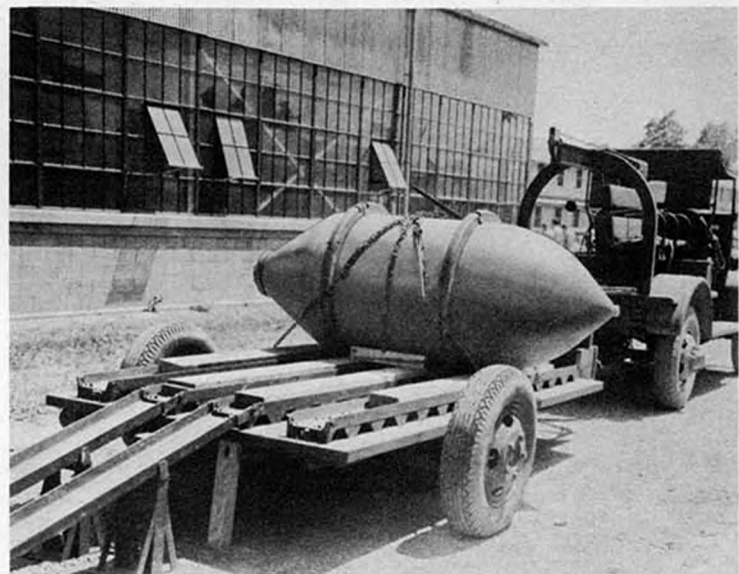
The bomb is blocked in front and rear and the dunnage is then nailed in place. The chains are placed around the bomb and held in place with the binders.
