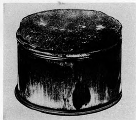
Fig. 77 - Effect of detonation on aluminum piston. Piston of aircraft engine showing the effect of severe and prolonged detonation through the use of improper fuel.
