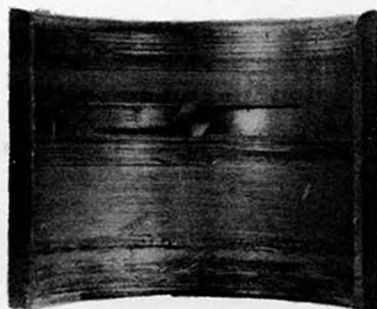
Fig. 20 - Bearing which has been badly wiped and scored because of lacking proper oil clearance.
