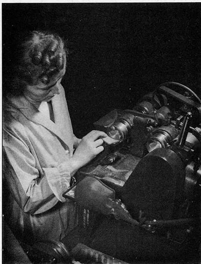
Centering cemented lenses on a lathe.
