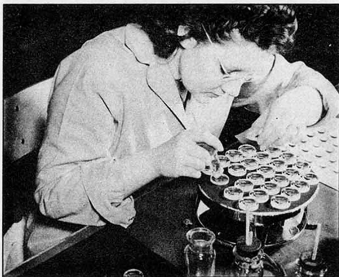
Cementing warmed lenses with Canada balsam.
