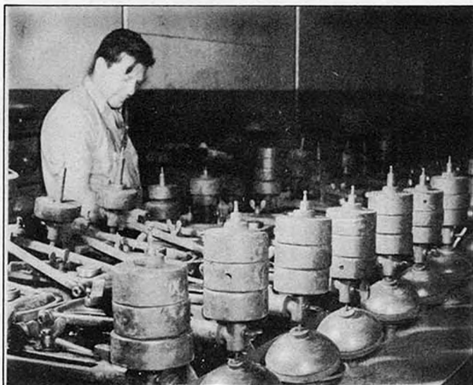
A battery of automatic polishing tools for finishing optical elements.
