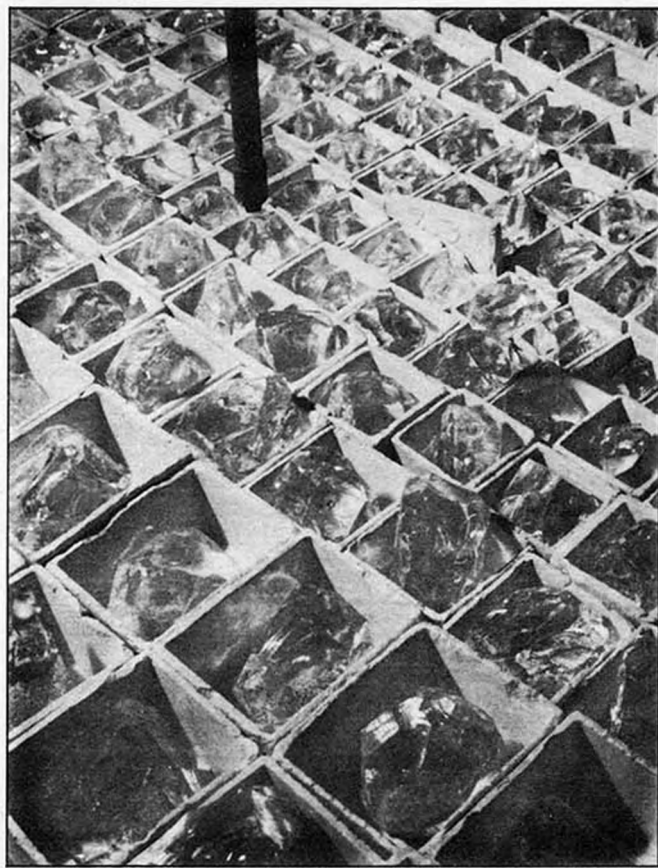
Chunk glass in fire-clay containers inside annealing oven.
