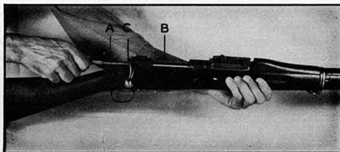
Figure 3 Rifle, U. S. Cal..30, M1903. (a) Gage, breech bore, (old) G2813, (b) Bolt special, G2813.
