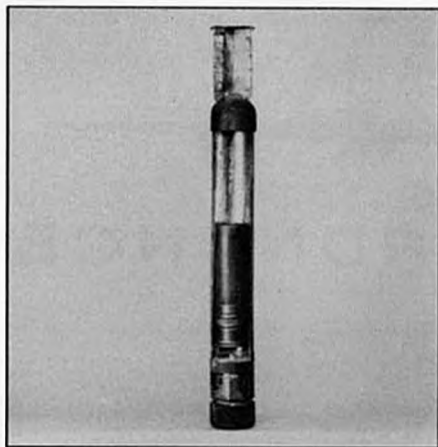
Photograph of the 8-ounce Mk I Incendiary Bomb of the World War. Note the heavy steel nose plug with the firing pin in its center. The 12-gauge shot gun shell filled with Thermit is resting on the two tin "ears", a close-up of which is shown below.
