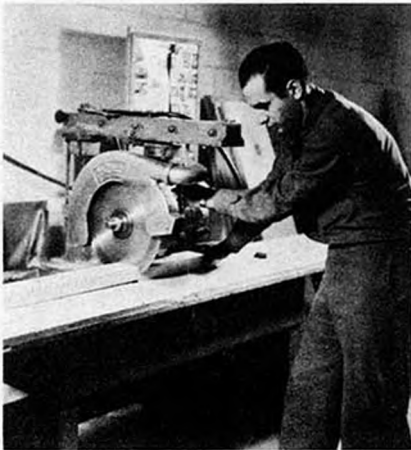
Figure 2 - Cut to length on the cut-off saw
