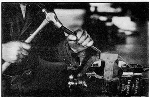
Bench Work - Chipping scale on cast iron block before filing. Use of simple hand tools in bench work considered important as an aid in developing feel and manual dexterity.
