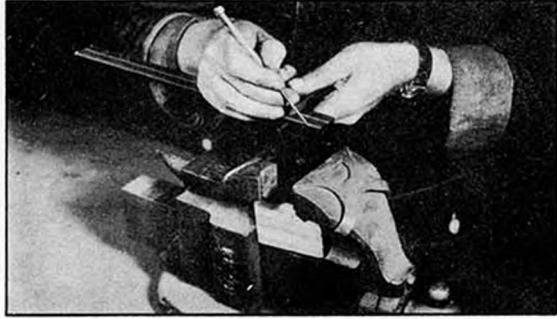
Bench Work - Simple lay-out of intersecting grooves on cast iron block prior to chipping and filing the grooves. Students work to an elementary mimeographed drawing.
