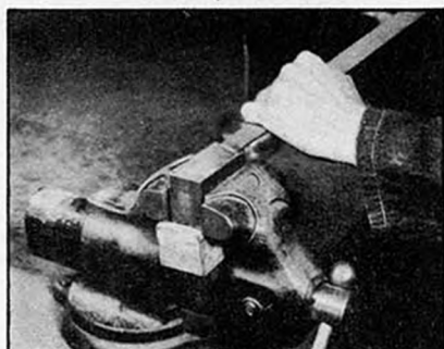
Bench Work - Scraping surface on cast iron block. Worn out files of different sizes and shapes ground smooth and sharp on end make excellent scrapers. Scraped surface is tested against surface plate.
