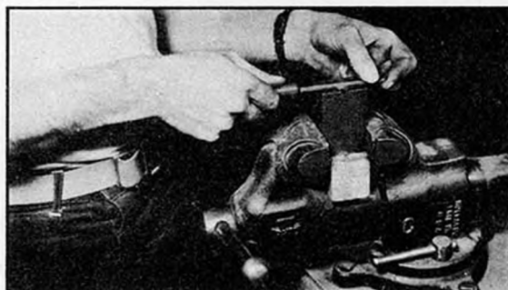
Bench Work - Filing grooves to a lay-out after chipping. Work required to be within 1/64 " of nominal size, narrow pillar file with safe edges used. Note packing block used under the work held in the vise to help support it.
