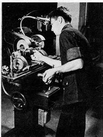
Advanced Milling- Sharpening teeth on milling cutter in a cutter grinder. An important operation, the life of the cutter and the quality of the work produced is influenced by the care and accuracy of this operation.
