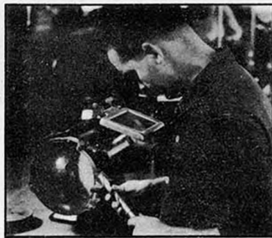
Bench Work - Off-hand sharpening of twist drill on bench grinder. The only method available for this operation if no drill grinder is available. Students drill holes in cast iron block after sharpening the drill. Note drill gage on bench near bench block.
