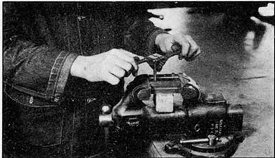
Bench Work - Tapping threads in cast iron block. 4 different types of thread are tapped for screws that require a counter-sink, a counterbore, a body size drill and fitting a pipe plug to a tapped hole.
