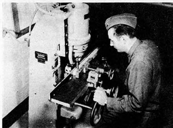
Figure 6 - "Drilling square holes"
