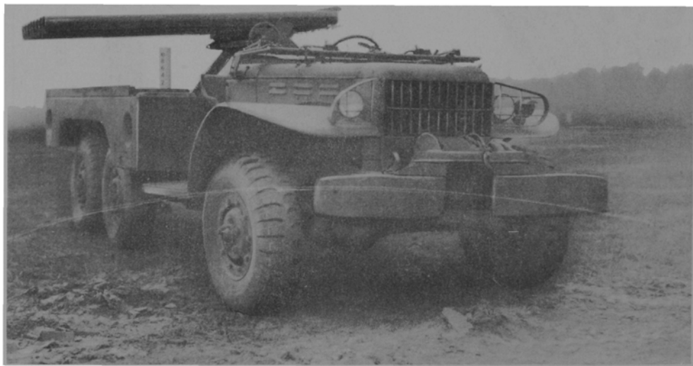
FIGURE 62. - T27 LAUNCHER MOUNTED ON 1-1/2-TON 6 X 6 PERSONNEL CARRIER. TOP: FRONT, 45° ELEVATION. BOTTOM: THREE-QUARTER LEFT FRONT, -5° DEPRESSION
