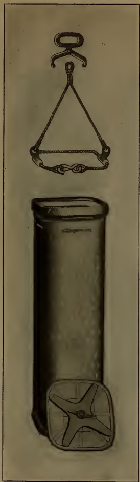
Fig. 38.—3"/50 Amm. Tank, Mk. II, with extractor.
