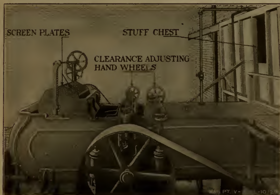
Fig. 9.—Duplex Beater, Pulping Machine.
