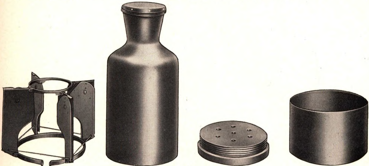
Figure 3.—Tail assembly, Propellant Chamber, Motor Base, and Shroud
