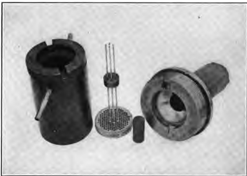
PLATE 31.—DIE BODY, PIN PLATE, PLUG, WATER JACKET, WATER-JACKET HEAD, AND SMOKELESS POWDER GRAIN FOR 12-INCH GUN.
