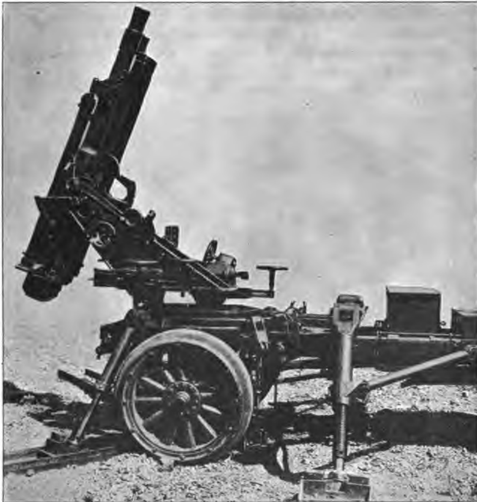
FIRING AND STABILITY JACKS.
