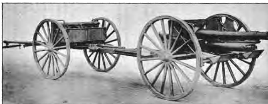
CARRIAGE AND LIMBER IN TRAVELING POSITION.
