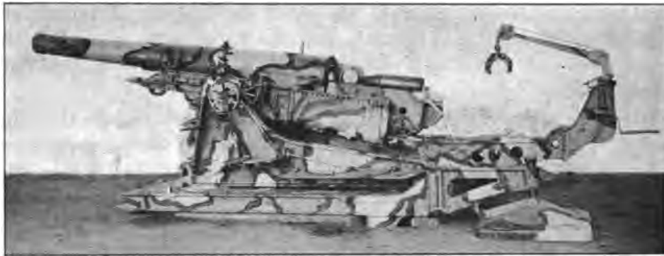
METHOD OF LOADING THE HOWITZER WITH RAMMER CAR.
