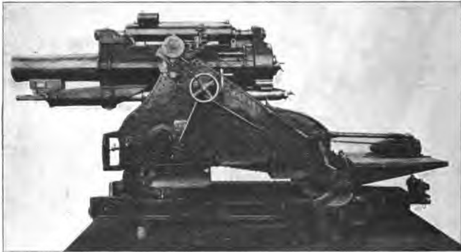
LOADING POSITION OF HOWITZER, SHOWING SHELL ON TRAY.
