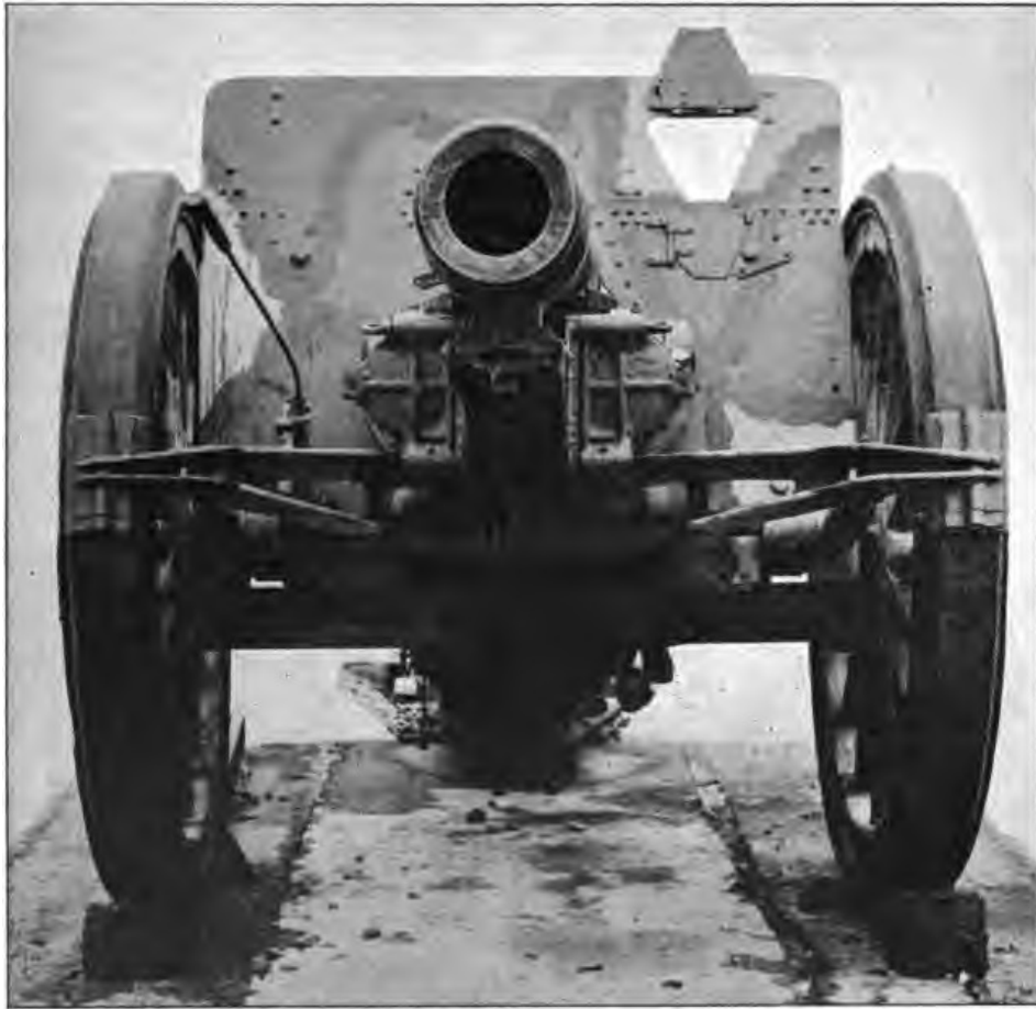
FRONT VIEW OF CARRIAGE EQUIPPED WITH TIRE BRAKES.
