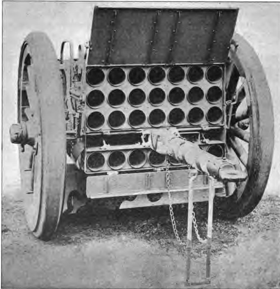
RIGHT FRONT VIEW SHOWING CHEST DOORS OPEN, EXPOSING DIAPHRAGMS.
