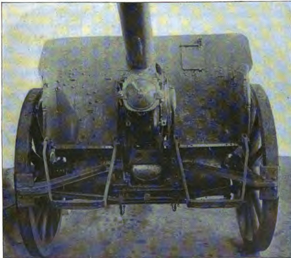
FRONT VIEW, SHOWING BRAKES AND TRAVELING LOCK.
