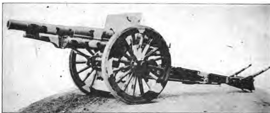
LEFT FRONT VIEW OF CARRIAGE EQUIPPED WITH BAND BRAKES.
