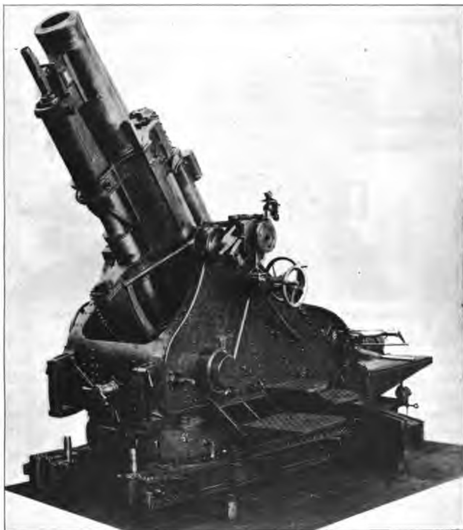
FRONT VIEW SHOWING MAXIMUM ELEVATION OF HOWITZER.
