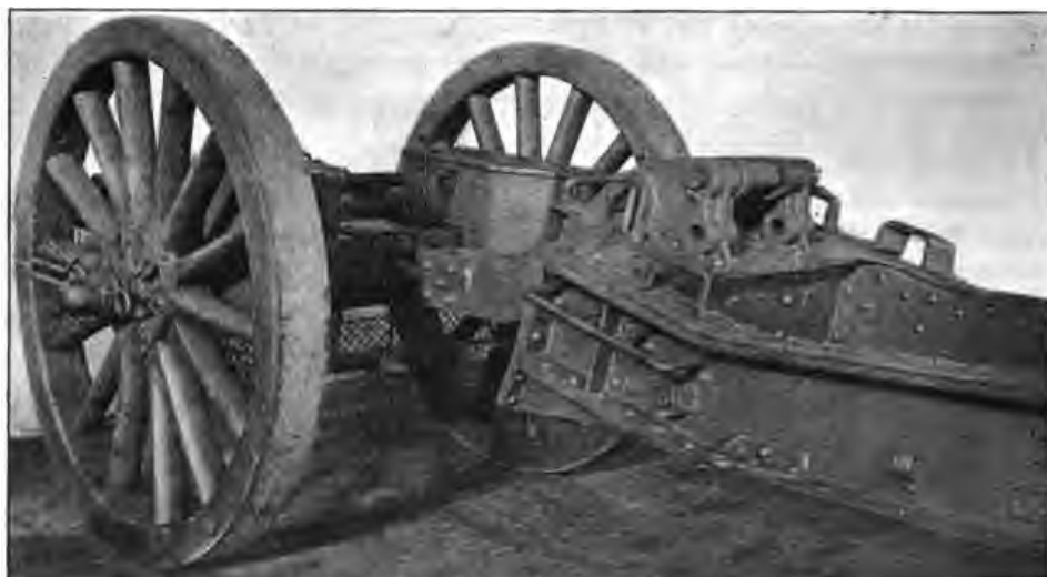
VIEW SHOWING TRAIL CONNECTED TO LIMBER.
