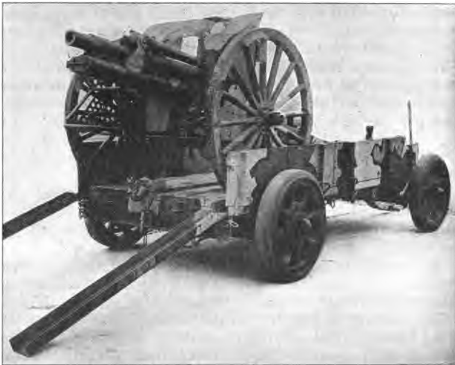
75-MILLIMETER GUN CARRIAGE MOUNTED ON A 3-INCH FIELD GUN TRAILER.
