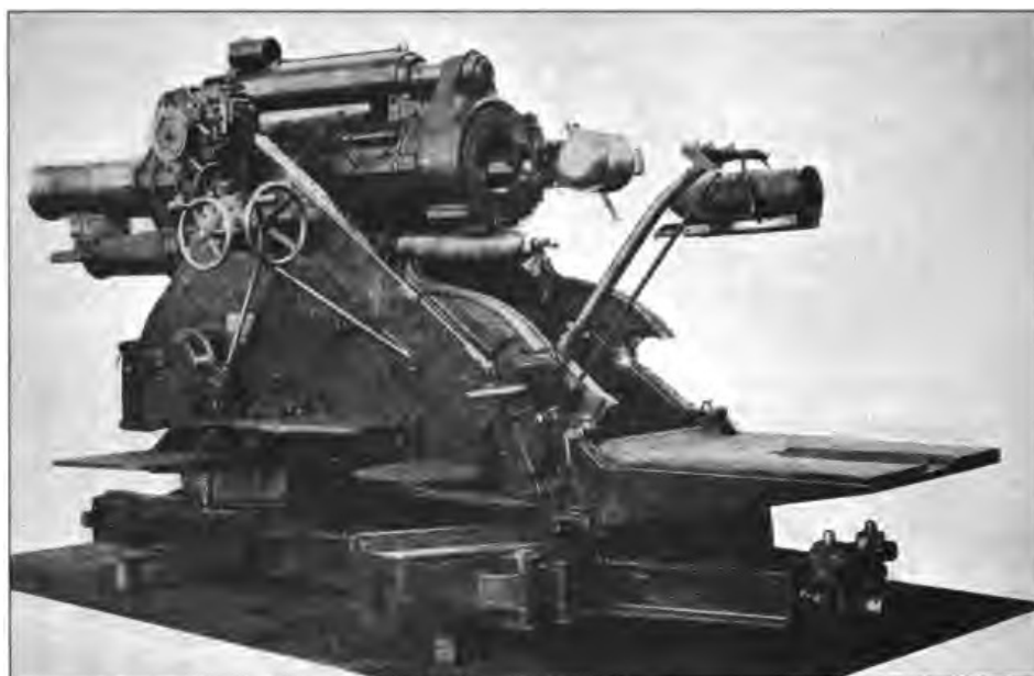
METHOD OF LOADING, SHOWING LOADING GEAR MECHANISM IN ACTION.
