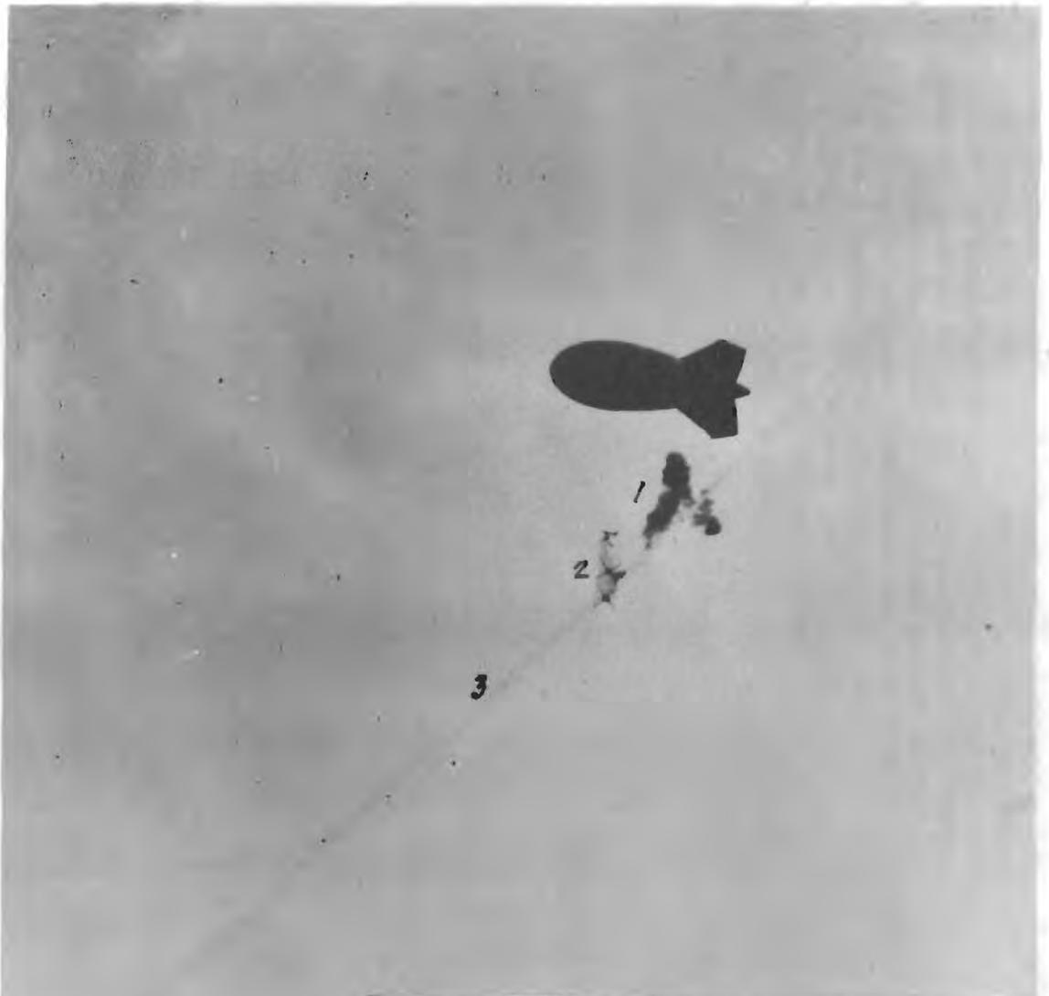
Fig.5. Operation of smoke puff, at 1, caused by the functioning of a radio proximity fuze as the antiaircraft rocket carrying it approached the balloon-suspended target at 2. The trajectory of the rocket is shown by the specially provided smoke trail 3. The smoke puff occurred after the rocket passed the target because of time-delay in the test squib used.
