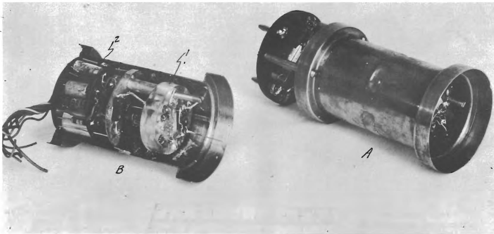
Fig.1. Radio proximity fuze unit used in field tests on bombs and rockets: A, assembled in unit container with switch plate at left; B, cut away to show the radio-frequency oscillator and diode assembly at 1 and the audio amplifier at 2. The entire unit excepting the radio-frequency coils is filled with polymerized tung oil to provide mechanical rigidity and shock mounting.
