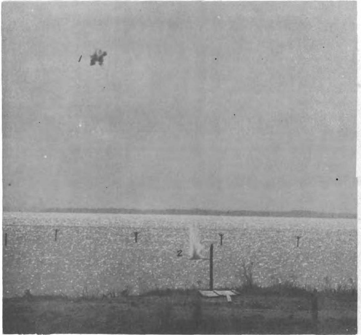
Fig.3. View showing operation of smoke puff, at 1, caused by the functioning of a radio proximity fuze as the bomb carrying it approached the sea. The splash of the bomb is seen at 2, near the target. The bomb was dropped from 10,000 ft and the fuze operated at 300 ft above the water.
