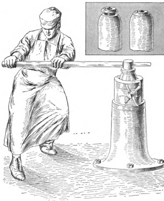
OPERATION 19. SCREW DOWN FUSE SOCKET
