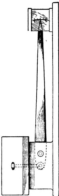
FIG. 640. MEASURING DEVICE FOR PRIMER ANVIL
