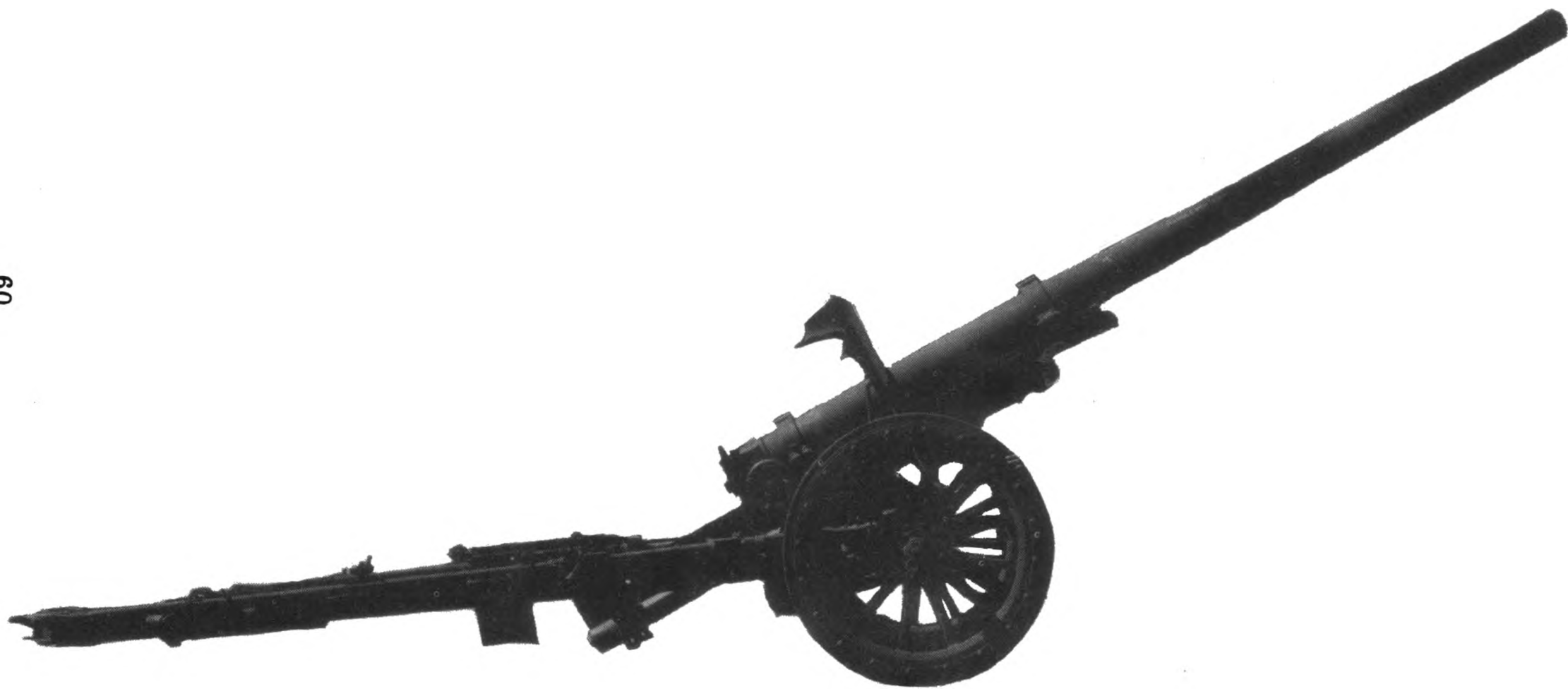
105 MM GUN, TYPE 92 (1932) Side view, with trails spread in position for high angle fire.
