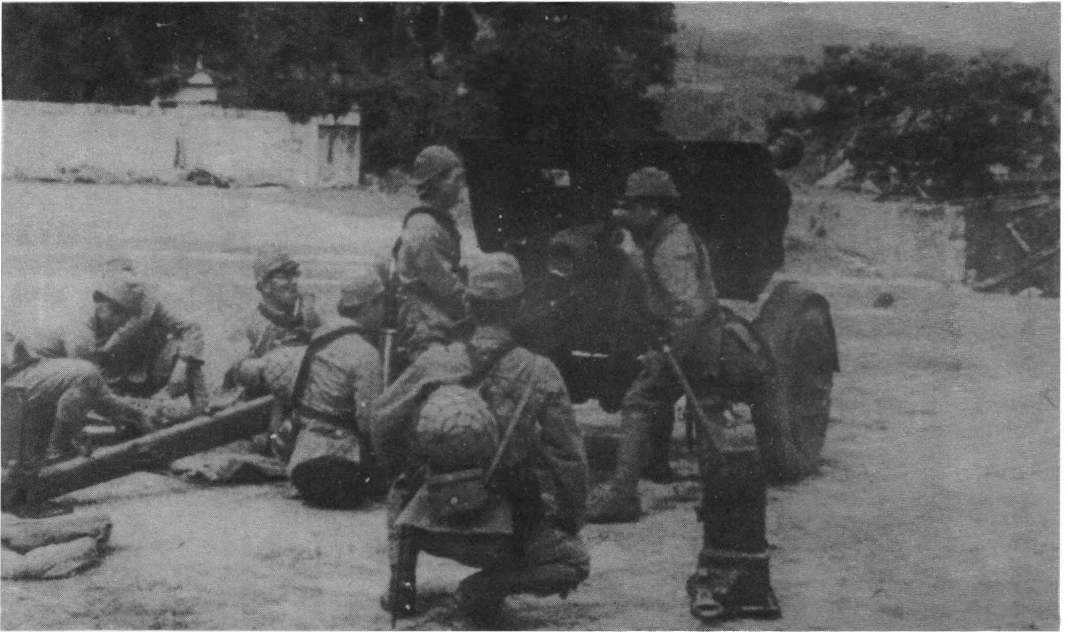
75 MM FIELD GUN, TYPE 90 (1930) Shown in position for firing
