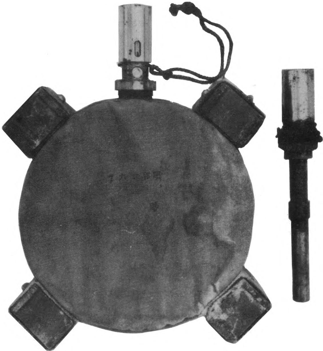
ARMOR PIERCING MINE (MAGNETIC) WITH FUZE SHOWN AT RIGHT
