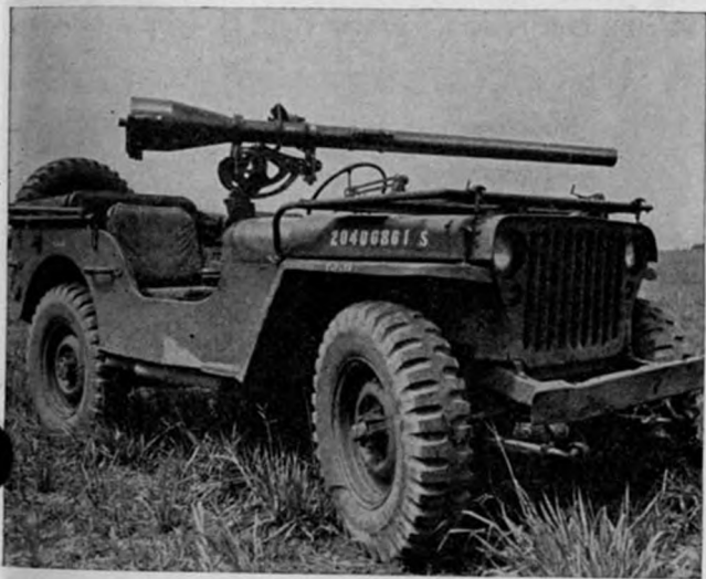
Figure 9. 75-mm rifle, M20, mounted on 1/4-ton truck, dashboard mount.
