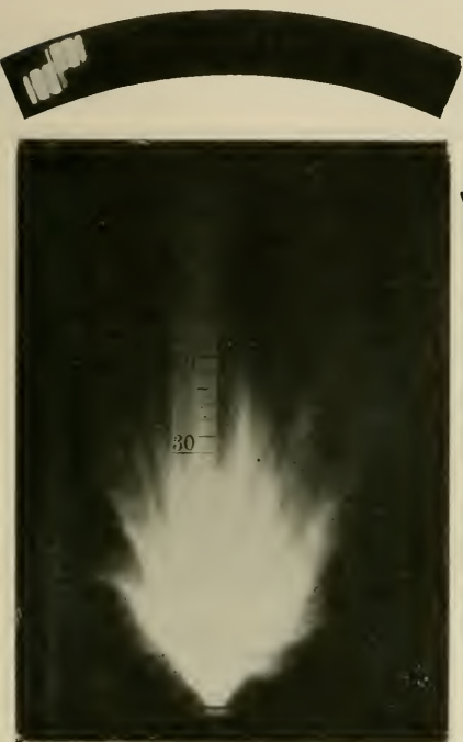
FIG. 136. Flame from Picric Acid with 5 per cent. Sodium Bicarbonate
