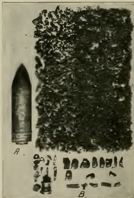
FIG. 122. 3-inch High Explosive Shell A. Recovered from sand butt after firing through a steel plate. B. Fragments resulting from high explosive bursting charge.
