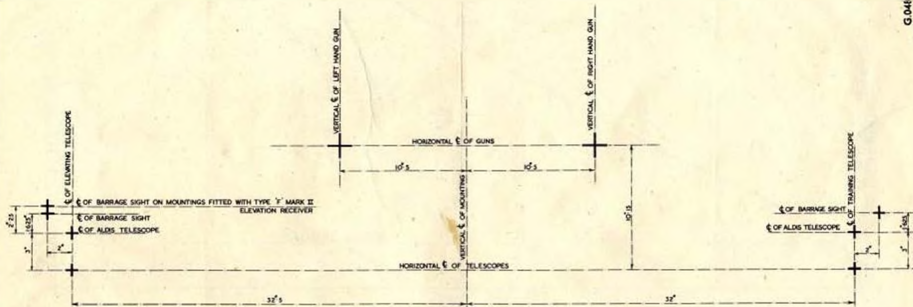
DIAGRAM A 4-INCH H.A. TWIN MOUNTING MARK XIX (INCLUDING R.P.50 SERIES) DIAGRAM OF SIGHT TESTING BOARD
