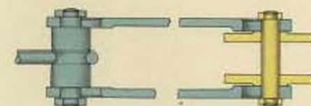
4" HA. MARK XIX MOUNTINGS ASSEMBLY OF REAR LINKS.
