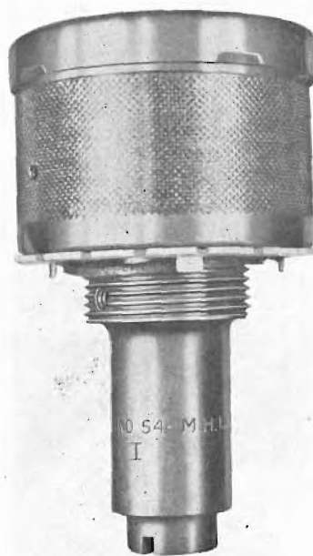
Fig. 1. The No. 54, Mk. I pistol
