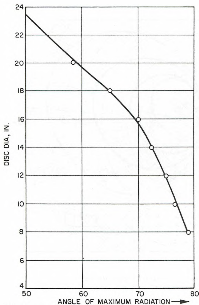
Figure 3-19 (S). Variation of Angle of Maximum Radiation for Change of Disc Diameter (U)
