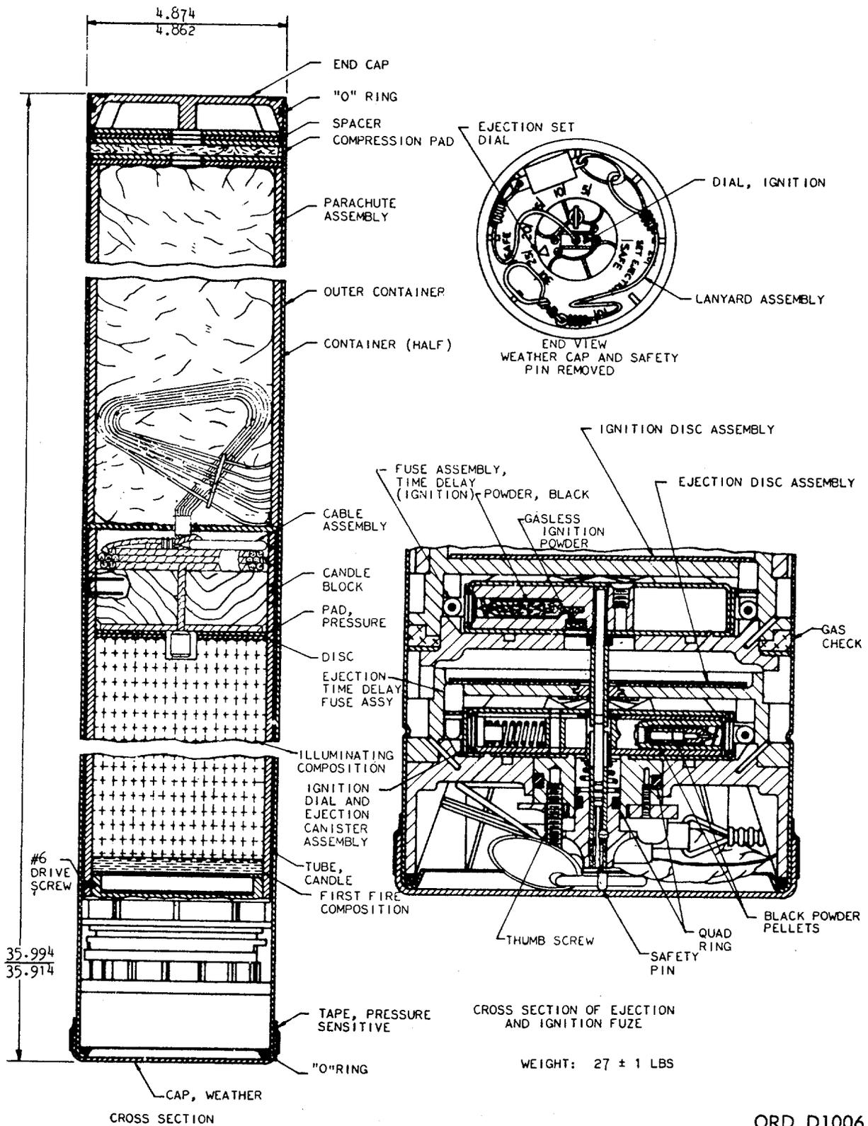
Figure 3-3. Aircraft parachute flare Mk24, mod 3.
