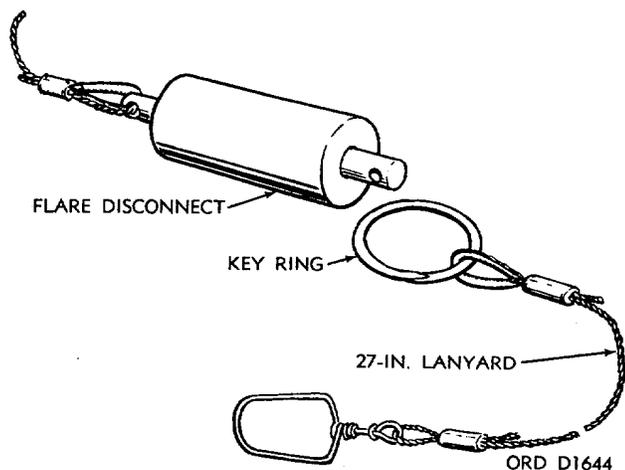
Figure 3-14. Removal of 27-inch lanyard and key ring.
