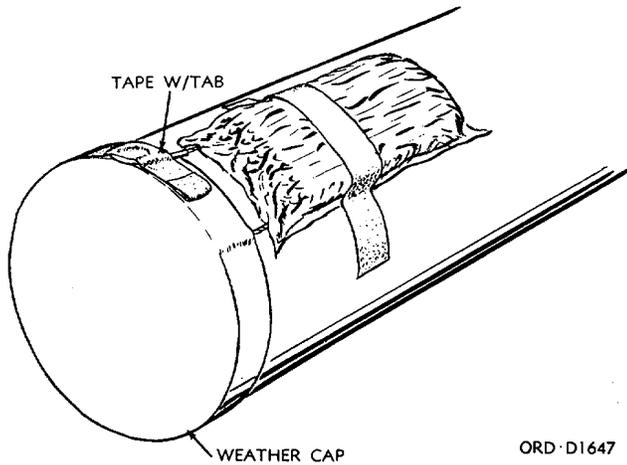
**Figure 3-17. Safety lanyard disconnect taped to weather cap.**
