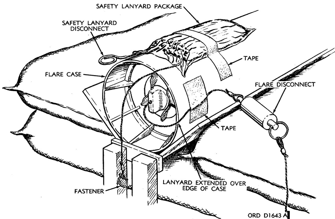
Figure 3-13. Positioning of flare in arming trough.
