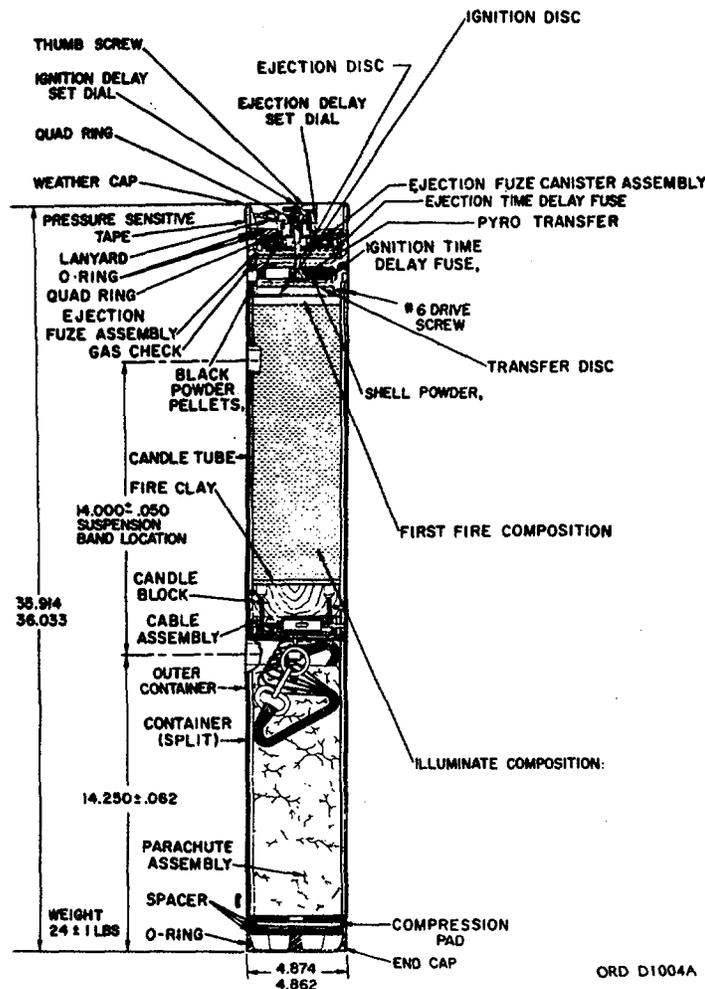
Figure 3-1. Aircraft parachute flare Mk24, mod 1.
