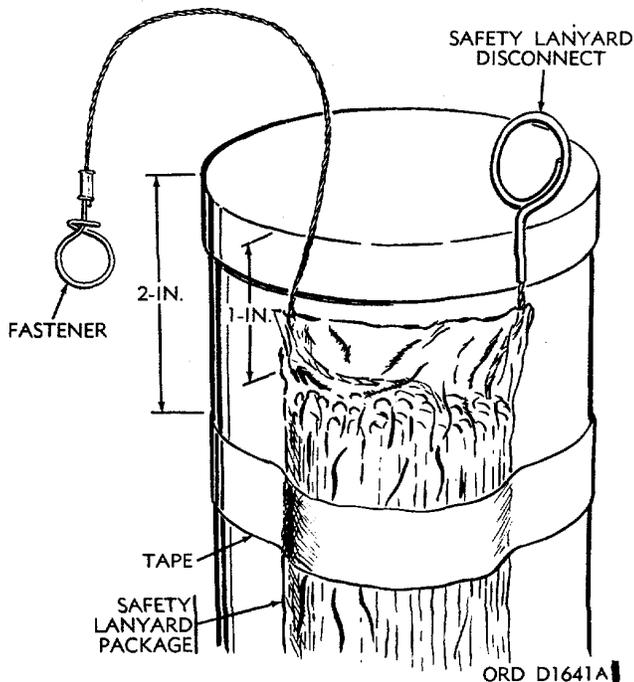
**Figure 3-12. Attachment of safety lanyard to flare case.**
