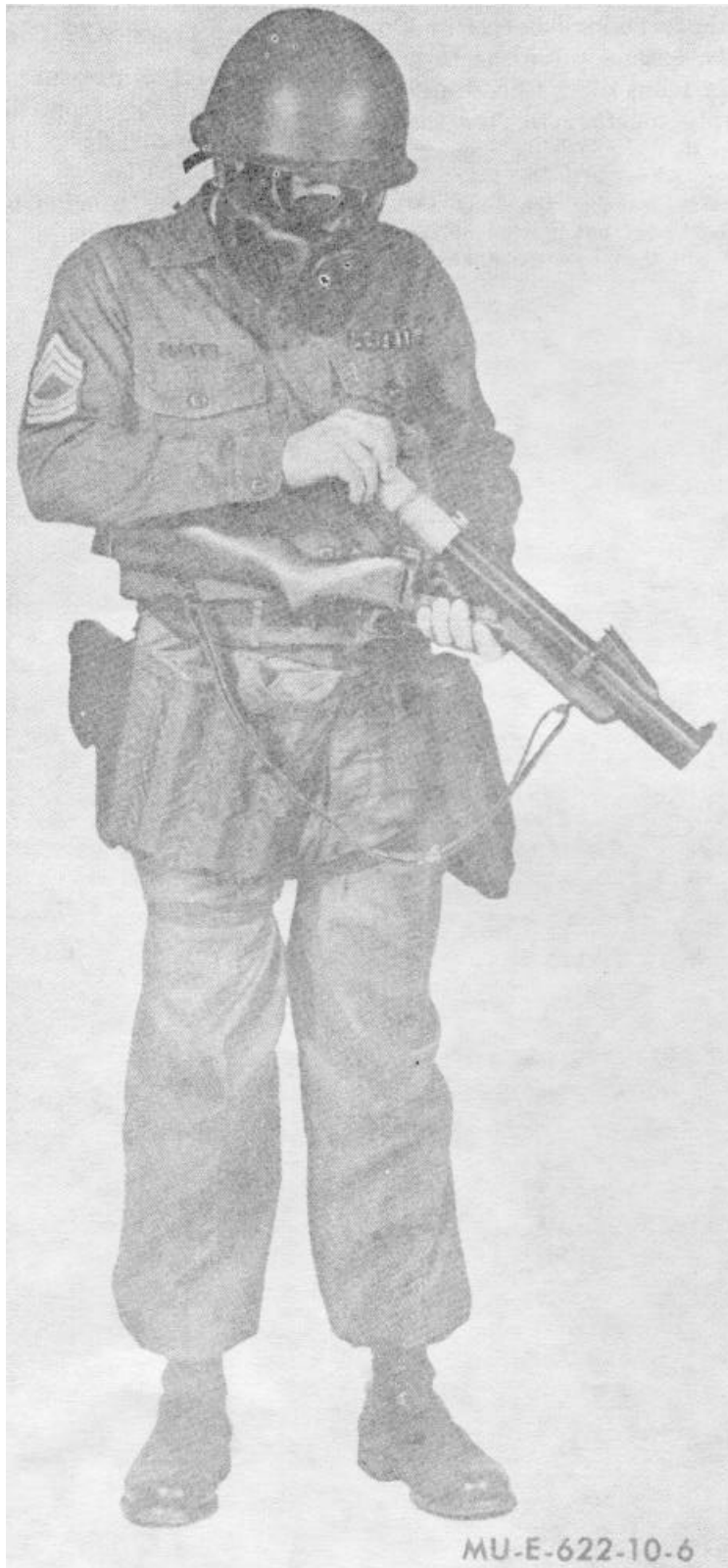
Figure 6. Loading cartridge into M79 grenade launcher (typical).
