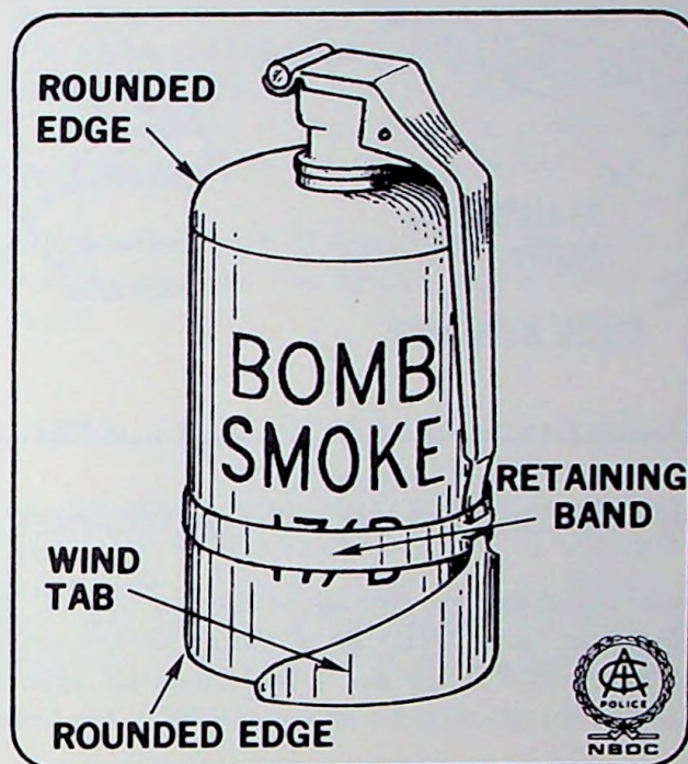
Figure 335 BLU-17/B BURSTING SMOKE WHITE PHOSPHOROUS (WP) BOMB
